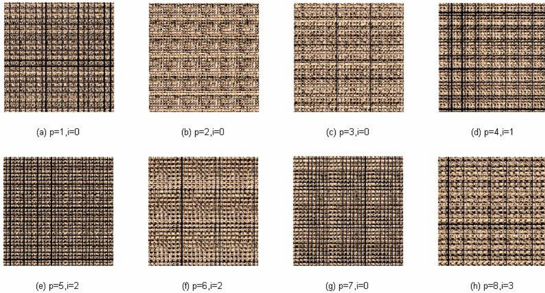
Fig. 4: Scrambled color image with different p and i value in spatial domain.
